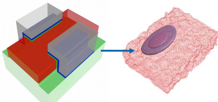
Models for two « face two face » quantum dots. On the left, finite elements model for the electrostatics (silicon in red, SiO<sub>2</sub> in green, HfO<sub>2</sub> in blue, and metal gates in gray). The metal gates control the potential in silicon; they can be used to trap, manipulate and « measure » electrons. On the right, atomistic model for the silicon wire, with the iso-probability surfaces of the first electron trapped under the left gate.
