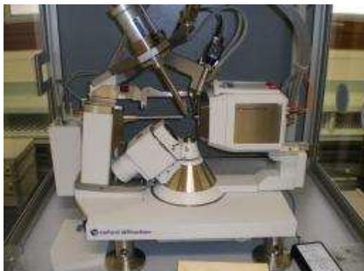
Rigaku XCalibur S (2008) equipped with a Molybdenum anode and a 4048x4048 pixels CCD detector. Nitrogen sample colling ( $T > 100\text{K}$ ) is available.
