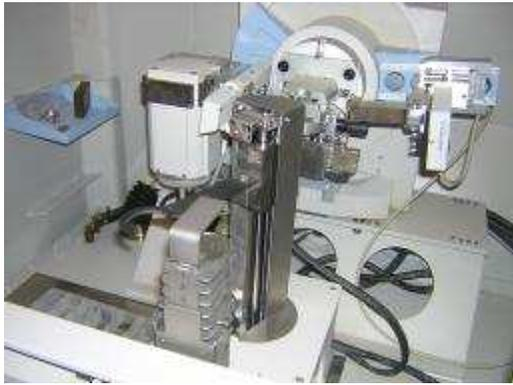
Upgraded in 2012, it is equipped with a copper anode, a 15 positions sample changer and an X'Celerator 1D detector. The diffractometer is mainly used in reflection Bragg-Brentano geometry with fixed or variable divergence slit. The sample holder can also be positioned in transmission mode especially for the investigation of membranes, with possibility to control the rotation angle in the sample plane.
