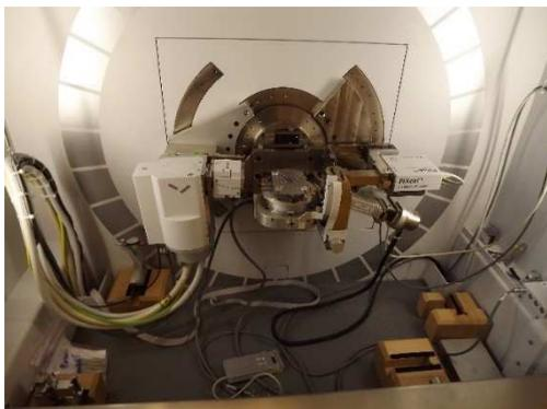
Diffractometer equipped with a cobalt anode (Co  $K_{\alpha 1}$  radiation prevents from fluorescence for samples containing iron and cobalt) and a chi, phi, z sample stage with RX, RY cradles for thin film alignment. It can be used in either diverging, parallel or mixed configuration.
